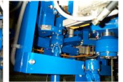
pic.5: Drive shafts with quick disconnect couplings
